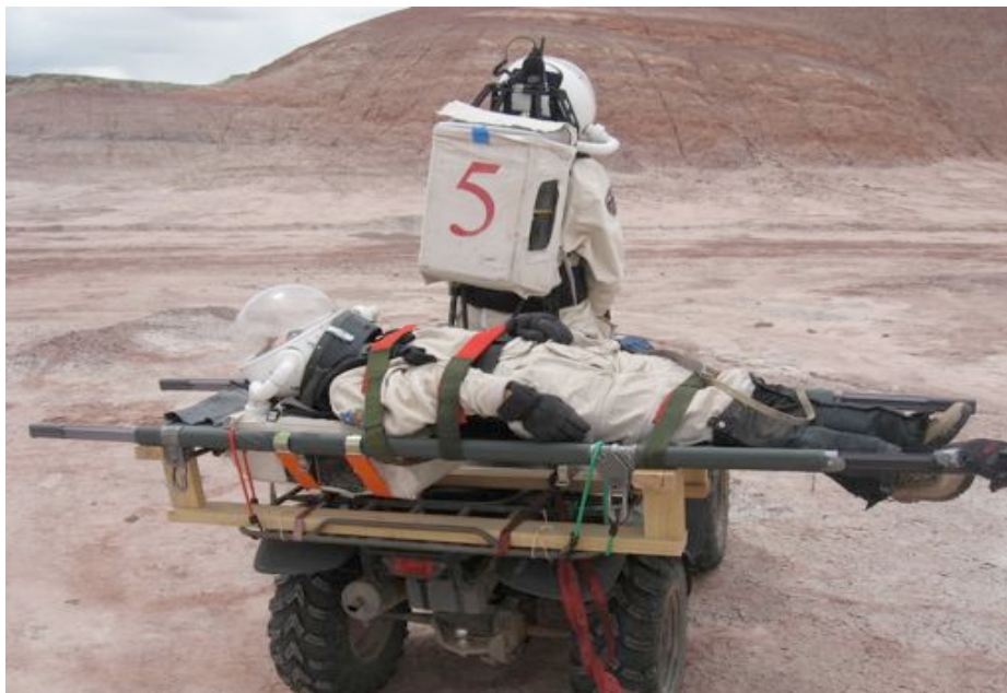
Figure 4. “Injured” crewmember being transported on the ATV-mounted stretcher.
