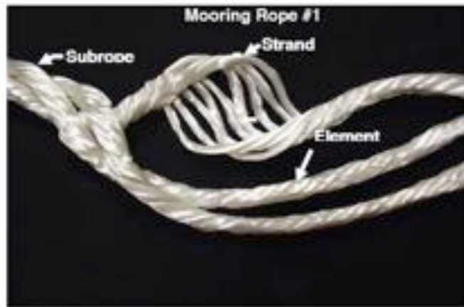
Figure 2 Definitions of strand, element and subrope (Mooring rope #1).
