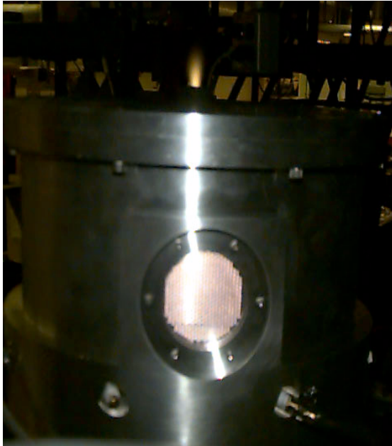
Figure 3. The 50kW, 915MHz MET thruster being run using air propellant. Second image shows its size relative to human being.
