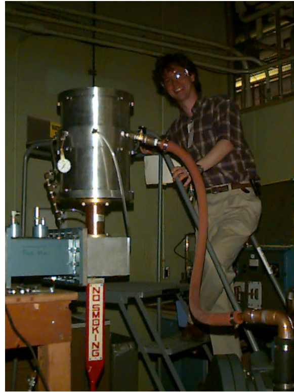
Figure 3. The 50kW, 915MHz MET thruster being run using air propellant. Second image shows its size relative to human being.
