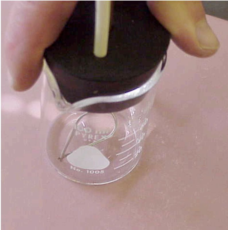
Figure 1. A stopper on a Mars Jar. This configuration will not work since the lip of the beaker prevents a seal from forming. The white tube on the stopper is an electrical feed through produced by running wire through a hollow plastic tube. The tube does not fit tight on the wire. 5 minute epoxy is used to fill the top end of the tube to seal the wire and the tube. The tube runs through a drilled stopper.
