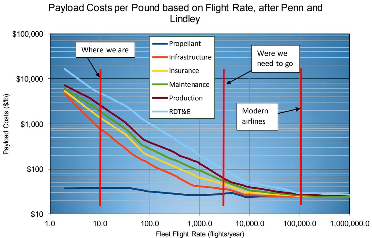
Figure 2 – Launch Cost Breakdown by Cost Driver and Launch Rate<sup>9</sup>
