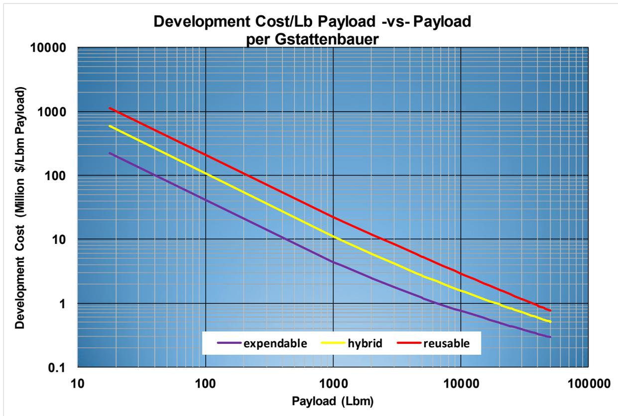
Figure 3 – Development Cost/Pound of Payload -vs- Payload Mass<sup>12</sup>
