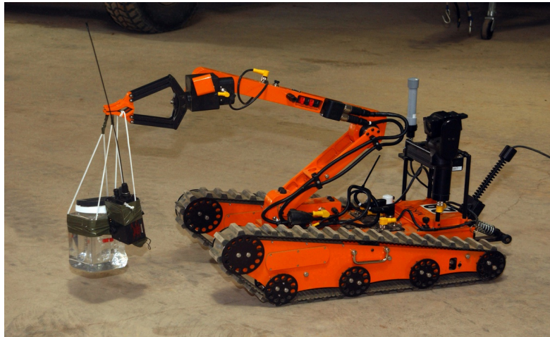
Figure 22: Navy EOD Robot which can be used as prototype for Base Cable and Piping (BCAP) Robot [51]
