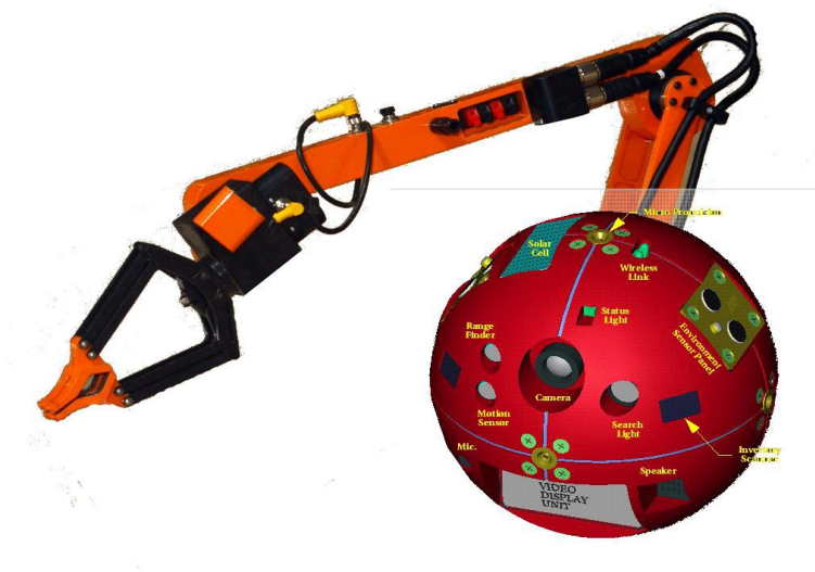
Figure 23: ISS SPHERES Robot which can be used as prototype for Stations Cable and Piping (SCAP) Robot[52]
