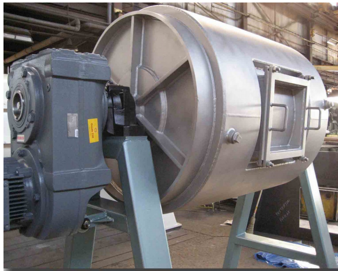
Figure 28: PATTERSON® 3'0" dia X 4'0" long batch type "DJ" Jacketed 304 Stainless Steel Ball Mill, with 10 HP Integral Gear Motor for dry grinding. This Mill has a special polished inside finish for a pharmaceutical application. Drive side view.[53]
